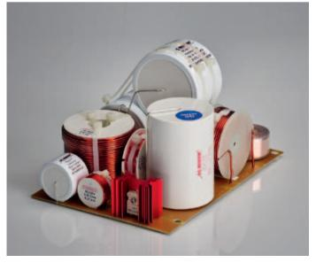
Surprisingly sparsely equipped for a 3-way crossover, only the best components are used for this. In front (on the red heat sink) the new Mundorf Super Resistors.
